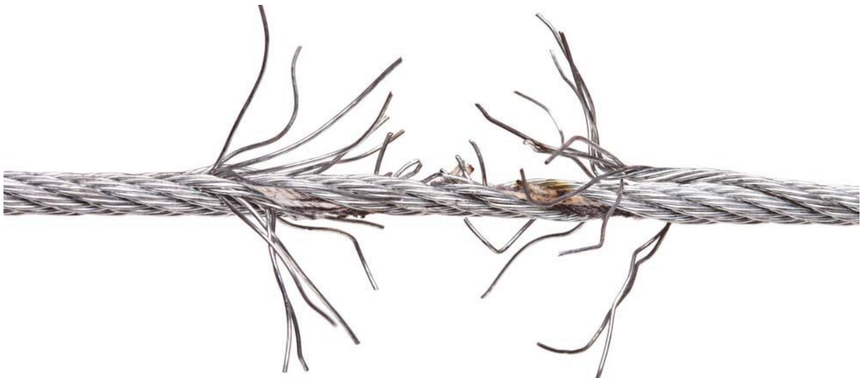
Figure 8.28 Damaged wire cable
